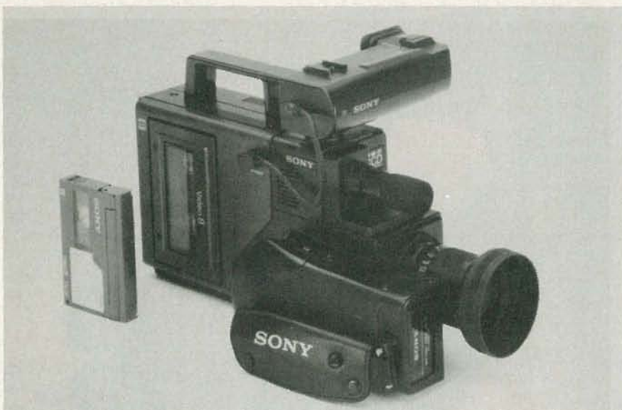
AN ALL-IN-ONE 8mm camcorder, the CCD-V8 from Sony can record two hours of video.
